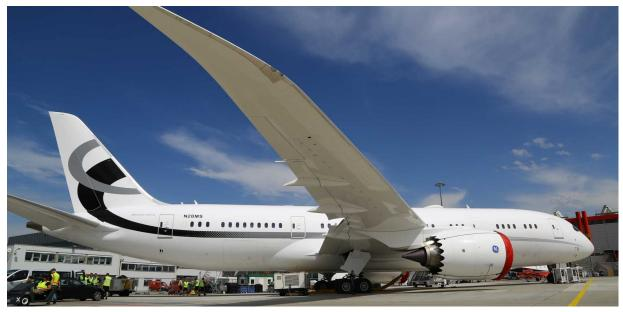
The 787 is also designed to ensure passengers arrive refreshed after journeys that may last as long as 16 hours, maintaining a 6,500-foot cabin at its 43,100-foot ceiling.
